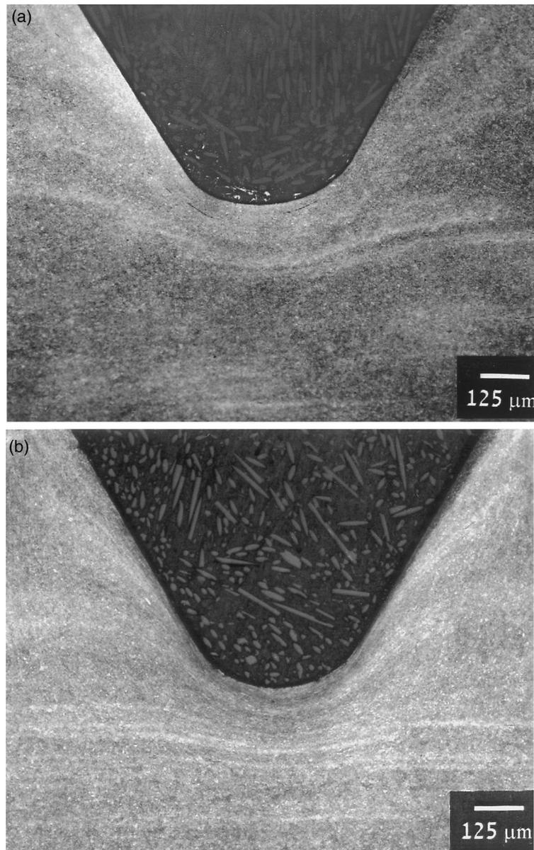
Fig. 3. OM micrographs showing the typical microstructure in the thread region of bolts: (a) cold-rolled before heat treatment; (b) cold-rolled following heat treatment; (c) machined before heat treatment; and (d) machined following heat treatment.
