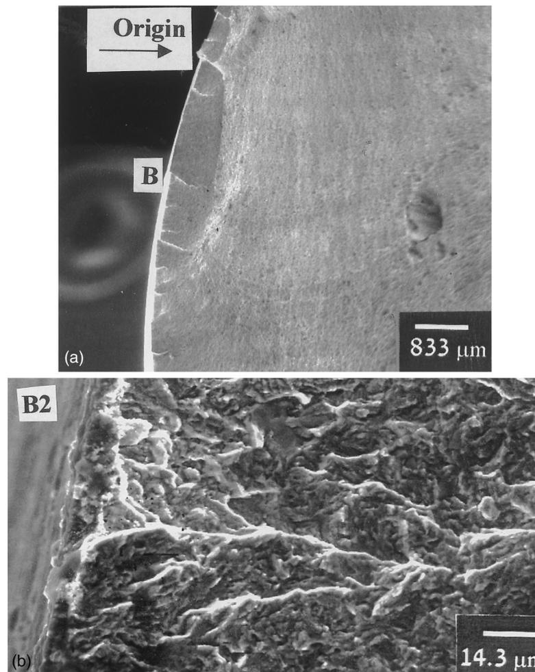
Fig. 2. SEM micrographs showing typical crack origin zone in a bolt from group HT/R following fatigue testing: (a) at low magnification; (b) at high magnification.
