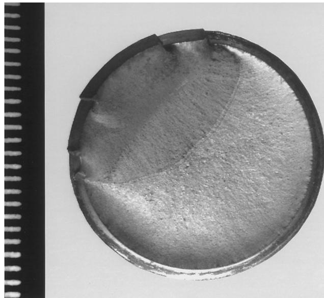
Fig. 1. Macroscopic view of fatigue fracture surface of a bolt from group HT/R. Similar fracture characteristics were observed for bolts from the other three groups.
